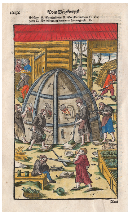
Glass furnace, with workers. Georg Agricola (German, 1494–1555). In De re metallica [Berckwerck Buch, Frankfurt-am-Main, 1580, p. cccxc]. Rakow Research Library.
